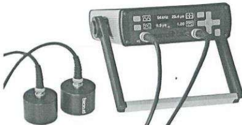
Figure II UPV Test Equipment
