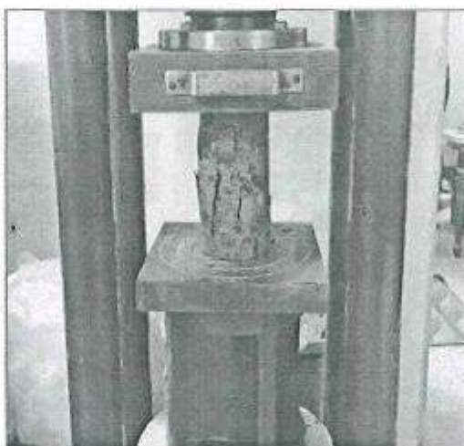
Figure VI Testing of Concrete Core
