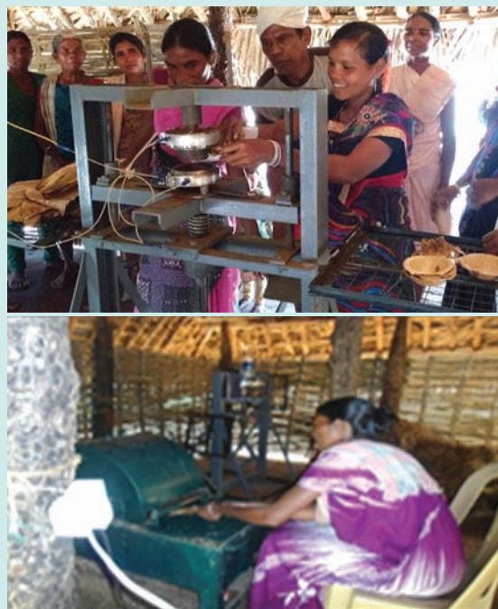
Bamboo Sheath Cup Making (Top) and Extraction of Palmyra Fiber
